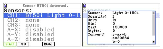
*Left: The CMA Light sensor BT50i is automatically identified. Right: The detailed sensor information is shown after selecting INFO.*
