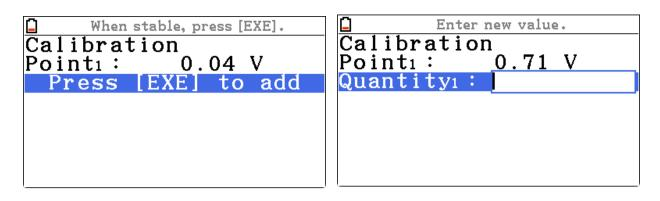
Left: The voltage for the calibration Point<sub>1</sub> is measured; accept its value with [EXE]. Right: The respective quantity value has to be entered.
