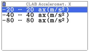
*Left: The internal accelerometer in the direction X is enabled. Right: The ranges available for the internal accelerometer.*  Please note that it is not possible to use different ranges for different accelerometer directions, the same range is used for all three directions.
