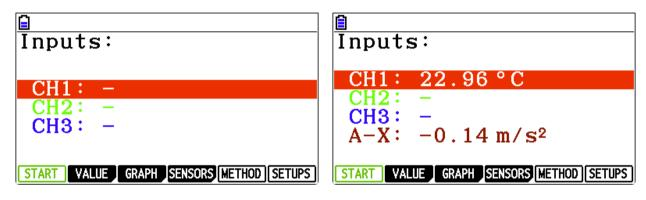
*Left: No sensors connected, no accelerometer axis enabled. Right: The temperature sensor is connected to input channel 1 and the accelerometer in X direction is enabled.*
