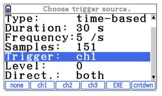
determine the state of the signal on the trigger channel to automatically start the measurement.
